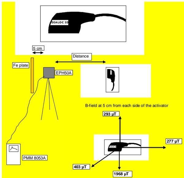
The B-field is especially high at the bottom side ( $\pm 21$  mT on the bottom and 2 mT at 5 cm) of the device and moreover it generates a substantial amount of harmonics
